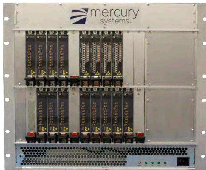
**Figure 1: Mercury's 48-channel, L-band direct digitization system**
